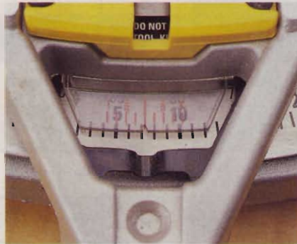
Above: Vernier scales on most saws give you \frac{1}{2}^\circ or \frac{1}{4}^\circ accuracy. The angle shown here is 7\frac{1}{4}^\circ .
